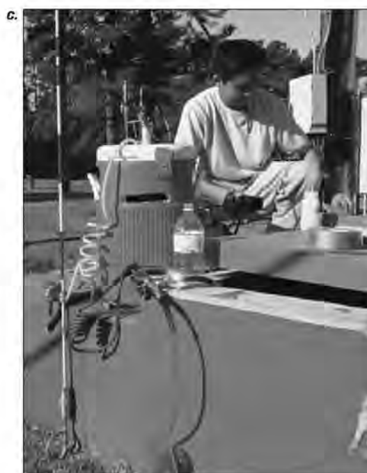
Figure I11. Method of connecting CRWQME to controlling storage tank: (a) schematic diagram, (b) photograph of connection to elevated storage tank SM-623, and (c) photograph of housing containing CRWQME and discharge tube, and staff person from U.S. Marine Corps Environmental Management Division. [See Figure I9 for location of storage tank SM-623; from Sautner et al. 2007; NPT, National Pipe Thread]
