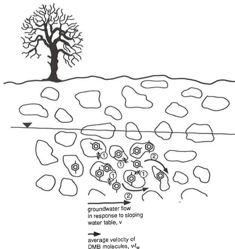
Figure 11.4 Illustration of the retardation of 1,4-dimethylbenzene (DMB) transport in groundwater due to: (1) reversible sorptive exchange between water and solids, and (2) limiting transport of DMB to that fraction remaining in the flowing water. As dissolved molecules move ahead they become sorbed and stopped, while molecules sorbed at the rear return to the water and catch up. Thus, overall transport of DMB is slower than that of the water itself.
