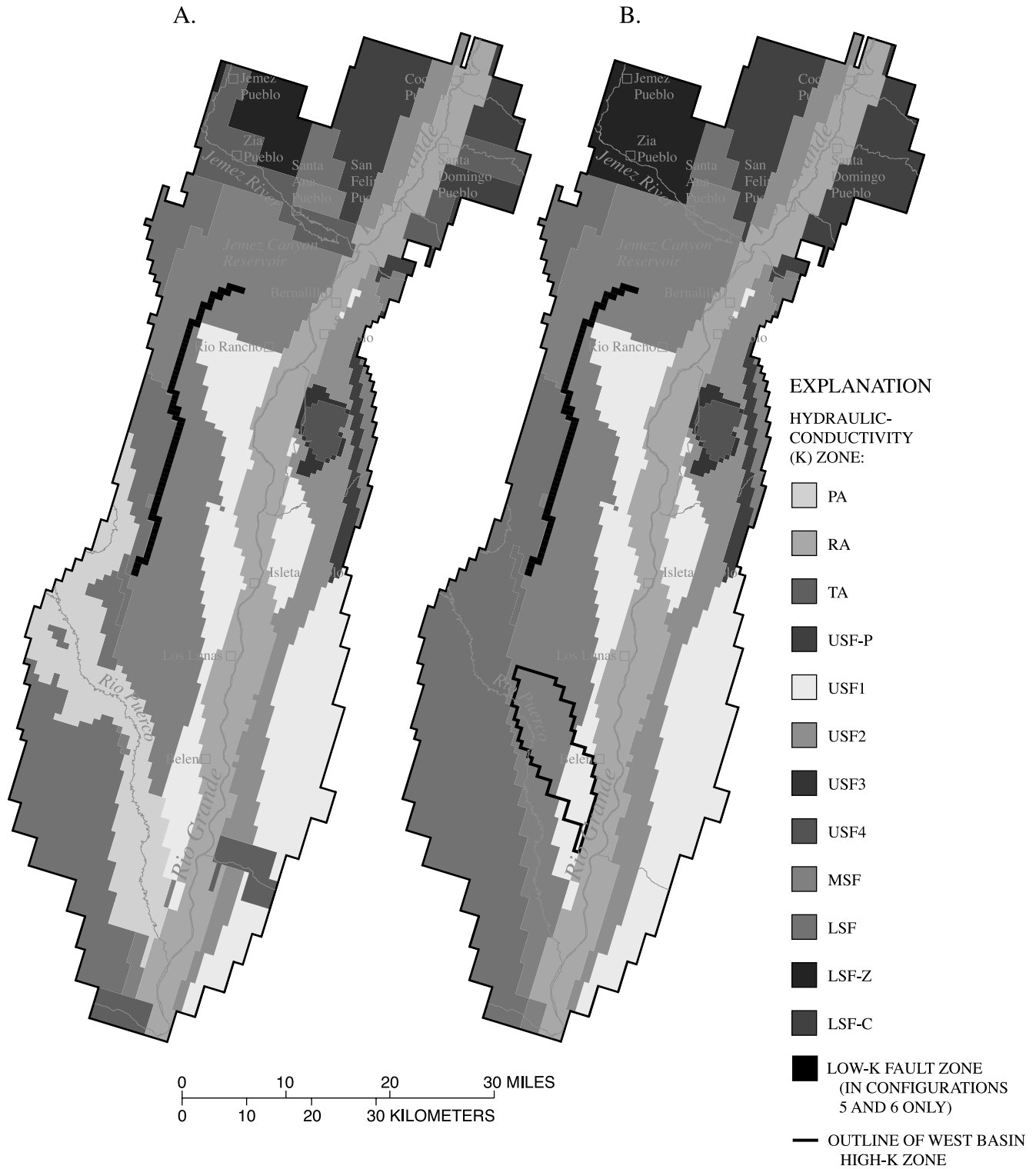
Figure 18. Hydraulic-conductivity zones identified for automatic parameter estimation in a ground-water flow model of the Albuquerque Basin, New Mexico: (A) zones in model layer 1, and (B) zones in model layer 2. (From Tiedeman and others, 1998.)
