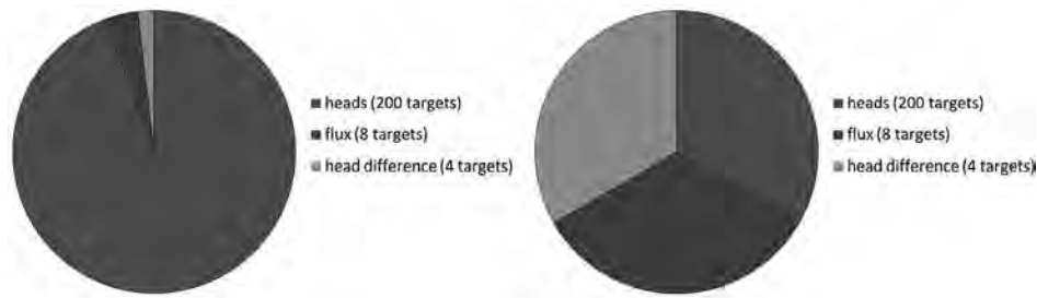
Figure B9.2.1 Pie charts of an initial objective function that is: (a) unbalanced because the number of head targets is much larger than other targets and (b) more balanced because no one target type dominates or is dominated by other groups. The more balanced objective function was obtained by simply normalizing the observation weights by the number of targets in each group.
