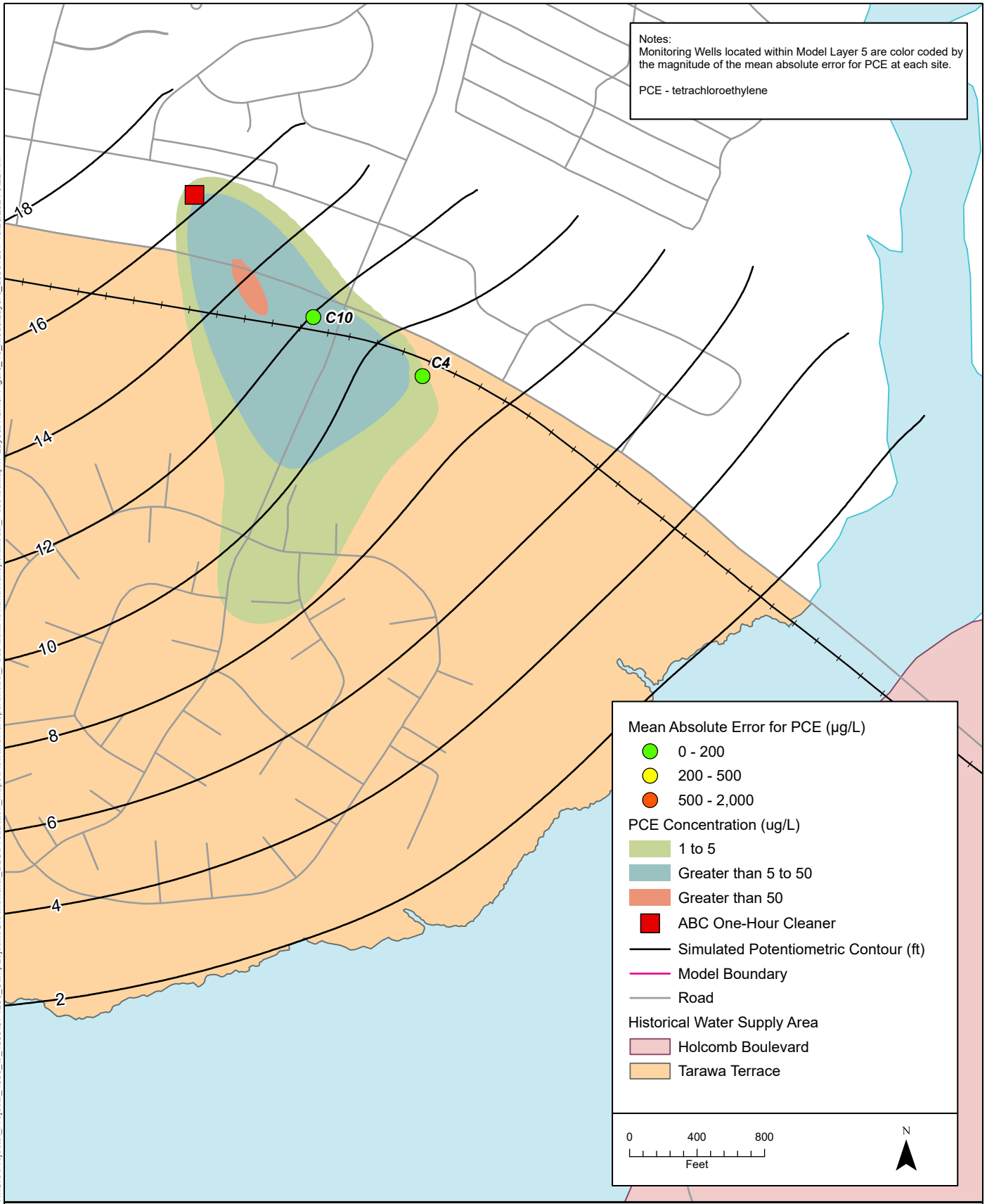
Figure 16. Simulated PCE Plume for December 2008 for Model Layer 5 Tarawa Terrace Flow and Transport Model Post-Audit
